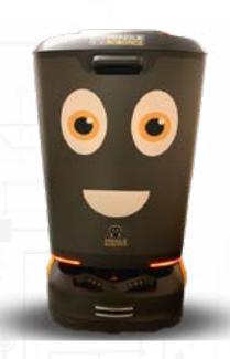
A time- and labor-saving solution was needed, and Pringle Robotics had the perfect one! "Dwight" the FlashBoT was installed and integrated with the hospital's elevator system to enable the robot to autonomously fetch patient specimens and transport them to the lab. The <a href="FlashBoT">FlashBoT</a> is an autonomous delivery robot that can only be opened using a passcode, ensuring that contents stay secure during transport.
